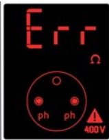
Connection between phases under 400V.
